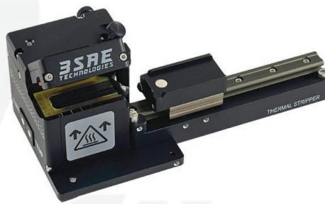
3SAE Thermal Strippers are compact, easy-to-use optical fiber stripping units designed to thermo-mechanically remove coatings from optical fibers.
