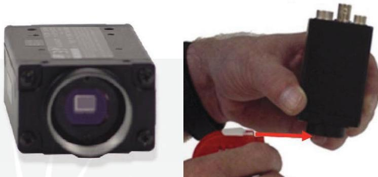
Blow air across and not directly at the CCD sensor of the camera.
