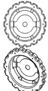
**DE8166:** 6 position MT-RJ insert with indexing
