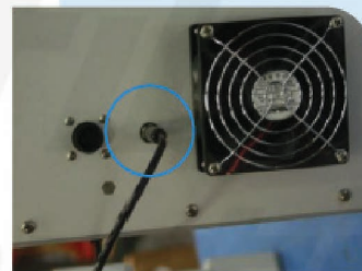
Figure 6. Connect Power Jack
