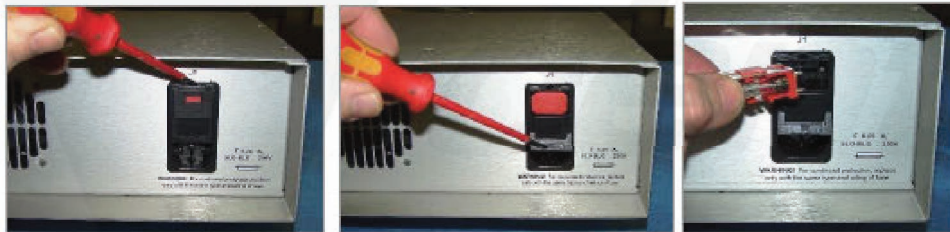
Figure 10. Replacing Fuses in the Power Supply
