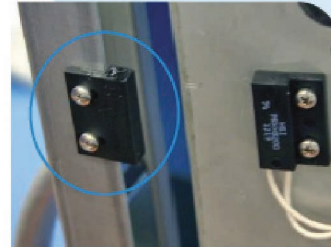
Figure 5. Install Magnetic Actuator
