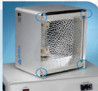
Figure 2. Remove Screws from Reflector
