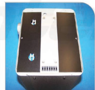
Figure 4. Two Temperature Control Plates Installed
