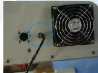
Figure 6. Connect Power Jack
