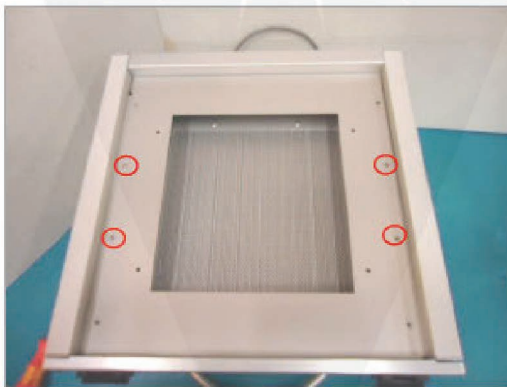
Figure 7. Remove Screws from Light Shield Top Cover
