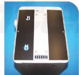
Figure 4. Two Temperature Control Plates Installed
