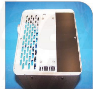
Figure 2. One Temperature Control Plate Installed
