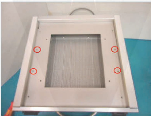
Figure 7. Remove Screws from Light Shield Top Cover
