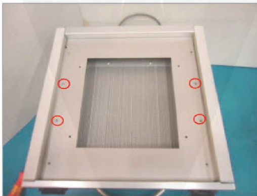
Figure 7. Remove Screws from Light Shield Top Cover
