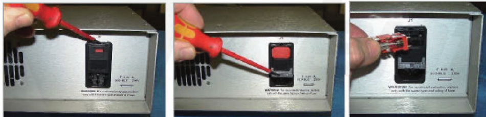
Figure 10. Replacing Fuses in the Power Supply
