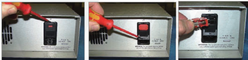
Figure 10. Replacing Fuses in the Power Supply
