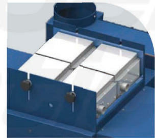
Four 5000-EC lamps full-width mounted 12" wide double exposure
