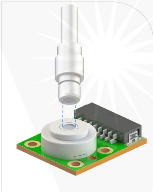
Figure 10. Aperture with 5-mm Lightguide
