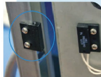
Figure 5. Install Magnetic Actuator
