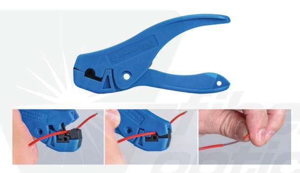
The Jonard Tools **BTR-6** Buffer Tube Ring tool provides quick access to fibers inside buffer tubes from 1.2 mm to 6 mm in diameter and will work with buffer tubes with wall thicknesses from 0.2 mm to 0.5 mm. The tool is light and durable with a hardened steel blade for long life and includes a hole for tethering.
