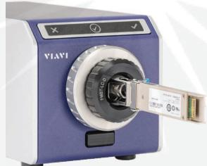
Technicians can leverage the FVAM-2000's built-in intelligence to streamline the fiber inspection process. By automating setup, tip configuration, testing, and data storage, it replaces the need for outdated manual devices. Simply attach the desired adapter and let the microscope handle the rest:
