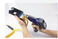
Inspect Duplex Connectors
