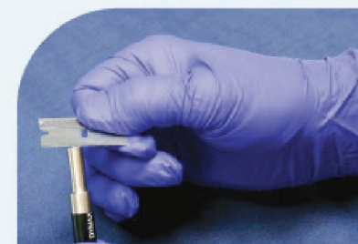
Figure 6. Clean Lightguide End With a Razorblade
