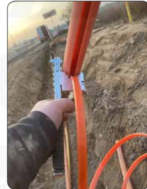
EASY FIBER DUCT SLITTER cuts a wide groove in the most commonly used duct types/sizes in one operation.
