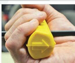
Close the tool onto the cable and pull in the direction of the arrow; clamps tightly — no latch required.
