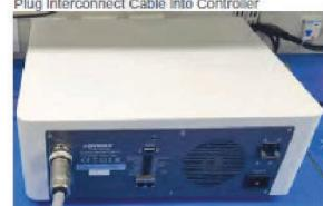
*Attention: When plugging in the female and male connectors, observe the key and keyway of each connector. The key should align with the keyway (Figure 14).*
