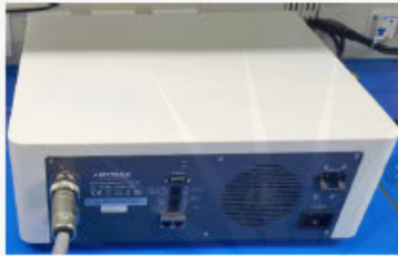
Figure 12. Plug Interconnect Cable into Controller
