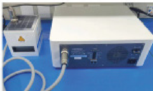
Figure 7. Interconnect Cable Installed
