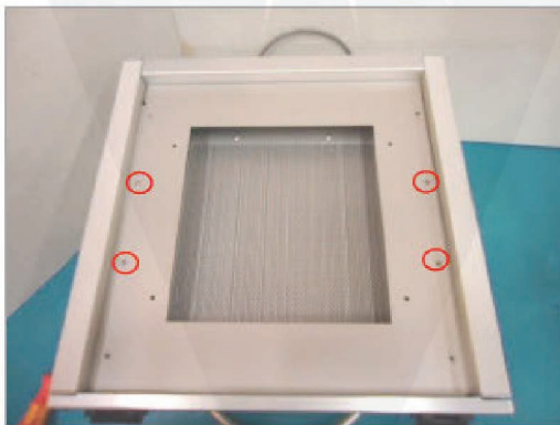
Figure 7. Remove Screws from Light Shield Top Cover
