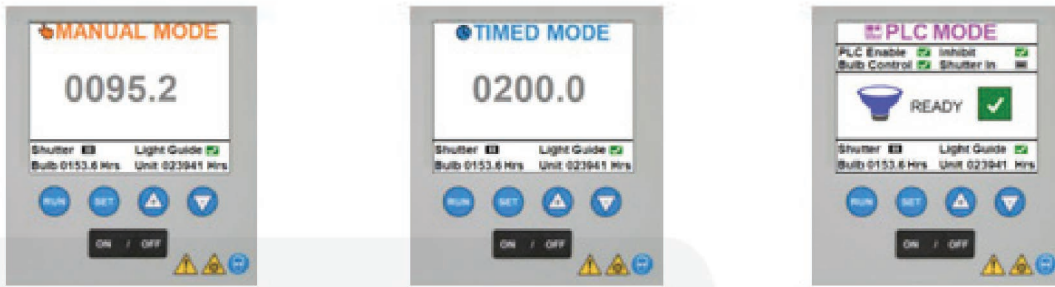
Figure 13. Mode Start-up Screens (Left to Right: Manual Mode, Timed Mode, PLC Mode)
