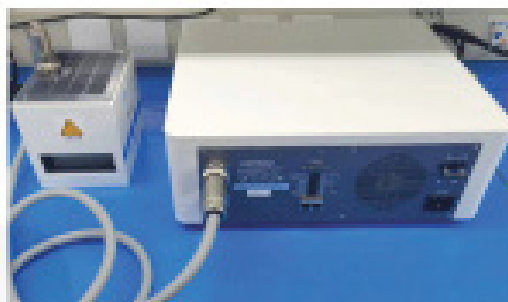
Figure 7. Interconnect Cable Installed
