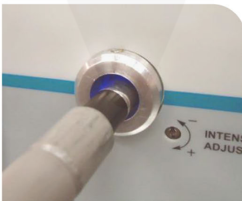
Figure 6. Insert Lightguide into Lightguide Mount
