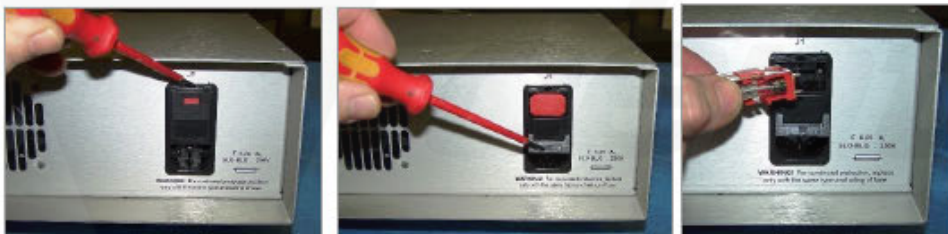
Figure 10. Replacing Fuses in the Power Supply
