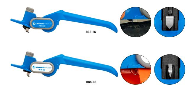
These ratcheting cable slitters are designed to dismantle heavy-duty cables. The RCS-25 and RCS-30 both slit and ring round cables greater than 1" (25 mm) in diameter, and the RCS-30 can also be used to make window cuts in ducts up to 5 mm thick. These slitters feature the following:
