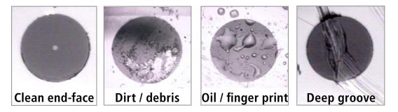
Loose contaminants (dust, dirt, etc.) and oil contaminants (grease, finger prints, etc.) can be removed with proper cleaning while permanent defects (pits, chips, scratches, etc) require a connector replacement. There are two types of fiber optic end-faces that need cleaning.
