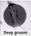
Loose contaminants (dust, dirt, etc.) and oil contaminants (grease, finger prints, etc.) can be removed with proper cleaning while permanent defects (pits, chips, scratches, etc) require a connector replacement. There are two types of fiber optic end-faces that need cleaning.
