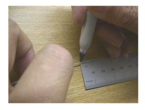
1.5 <u>Strip Buffer:</u> Strip 1.75 inches of buffer from the fiber using a Micro-Strip tool with properly matched bushing and blades. Be very careful not to damage or scratch the sides of the fiber. Please refer to fiber manufacturer's recommendations for the proper blade and bushing for MicroStrip tool.
