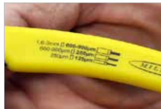
Convenient stripping guide printed on the tool handle.
