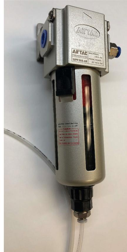
Replacement Filter Elements are Domaille Part# **PM22399**. Install the new Filter Element and lightly tighten with the wrench. Reinstall the Filter Bowl at 45° and turn to engage the latch. Reconnect the air supply.
