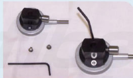
Figure 5. Attach Lightguide Adapter to Lightguide (Step 4)
