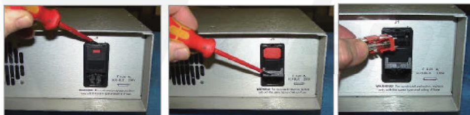
Figure 10. Replacing Fuses in the Power Supply
