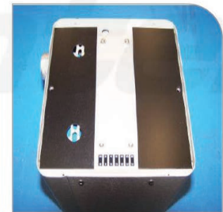
Figure 4. Two Temperature Control Plates Installed
