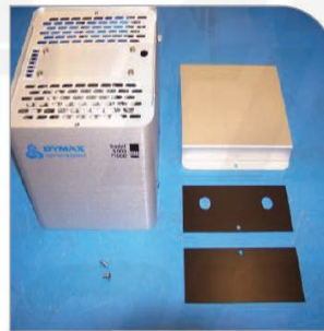
Figure 1. 5000-EC with Cover Removed & Temperature Control Kit
