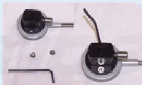
Figure 5. Attach Lightguide Adapter to Lightguide (Step 4)
