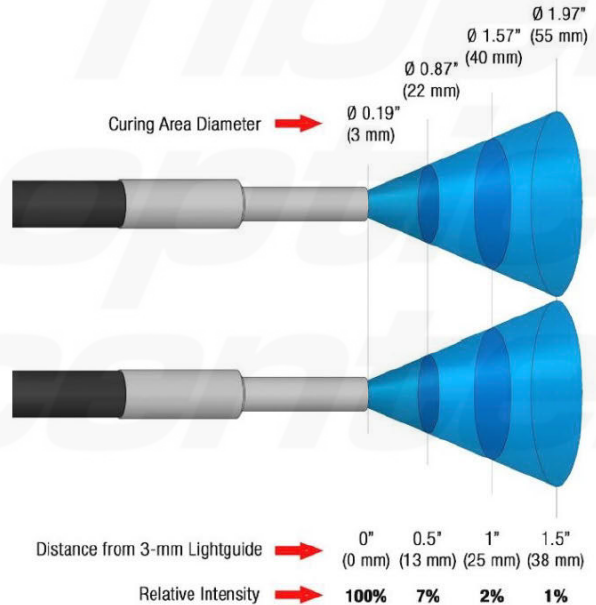
Figure 3. Curing Area/Intensity vs. Distance Using a 2-Pole, 3-mm Lightguide
