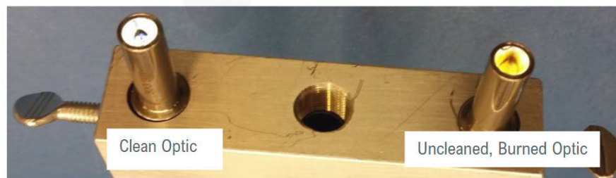
Figure 4. Damaged, Burned Lens
