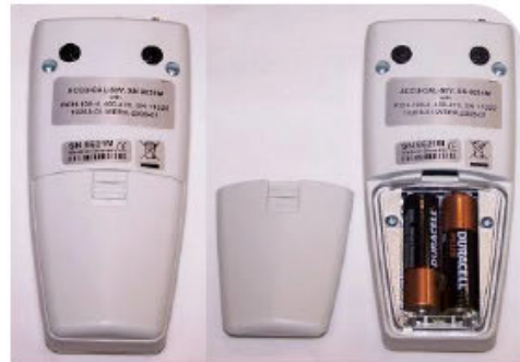
Figure 7. Battery Compartment (Closed & Open)
