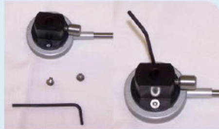
Figure 5. Attach Lightguide Adapter to Lightguide (Step 4)
