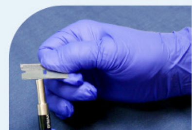
Figure 6. Clean Lightguide End With a Razorblade
