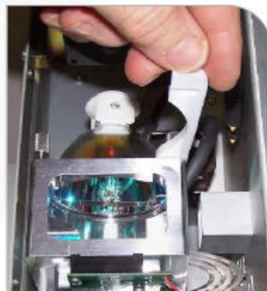
Figure 3. Lift Bulb Mounting Bracket
