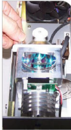
Figure 11. Tighten Mounting Bracket Thumbscrews
