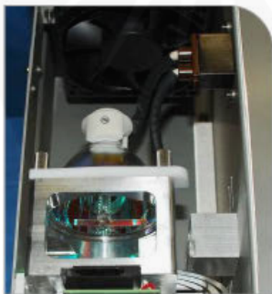
Figure 2. Bulb Installed in Bulb Mount
