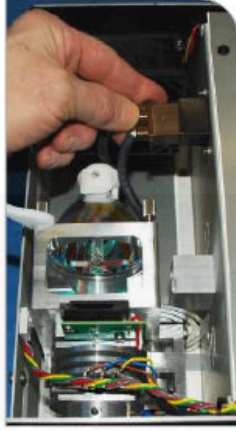
Figure 10. Plug in Bulb
