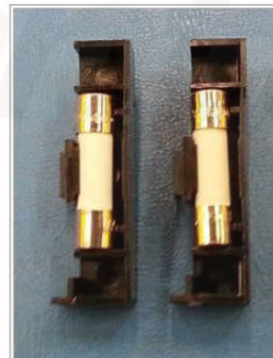
Figure 52. Fuses Removed from Holder
