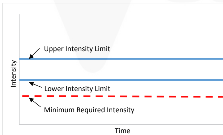
Figure 2. A Controlled UV Flood-Curing Process
