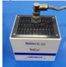
Figure 13. Plug Interconnect Cable into Emitter
