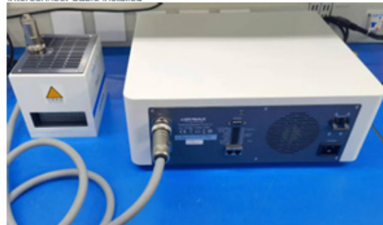
Figure 7. Interconnect Cable Installed
