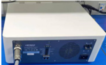
Figure 12. Plug Interconnect Cable into Controller
