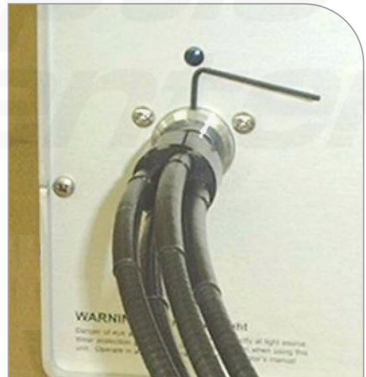
Figure 2. Tighten Set Screw with Hex Wrench
