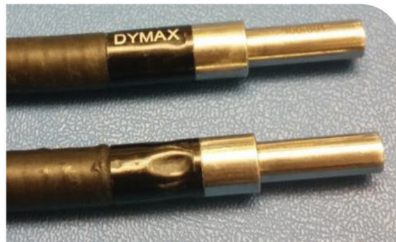
Figure 8. Damaged Lightguide Caused by Over Tightening
