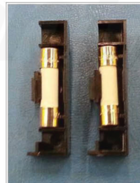
Figure 52. Fuses Removed from Holder
